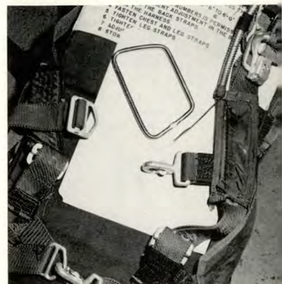
Above, "hot" wires in this uncovered switch panel burned the ripcord cable of the chute, below, and "D" ring slipped completely free.
