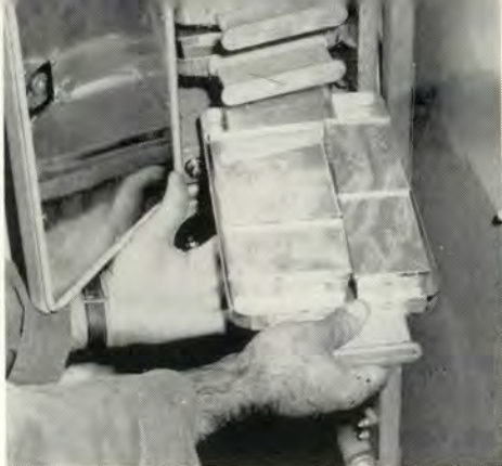
Meals are precooked on the ground then heated during the flight in the airborne oven.
