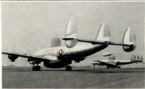
The black radome on the Super Snooper's belly holds a revolving antenna, while the fin-like protuberance houses additional radar.
