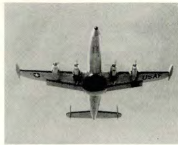
EC-121 flying radar stations are patrolling our shores on a 24-hour basis. Extra fuel in the tiptanks gives added range and endurance.
