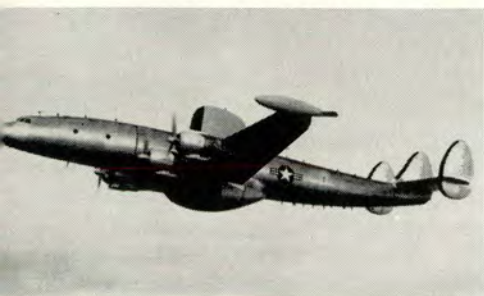
EC-121 flying radar stations are patrolling our shores on a 24-hour basis. Extra fuel in the tiptanks gives added range and endurance.
